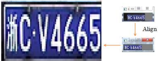
(Fig2. The extracted plate before and after Alignment)
