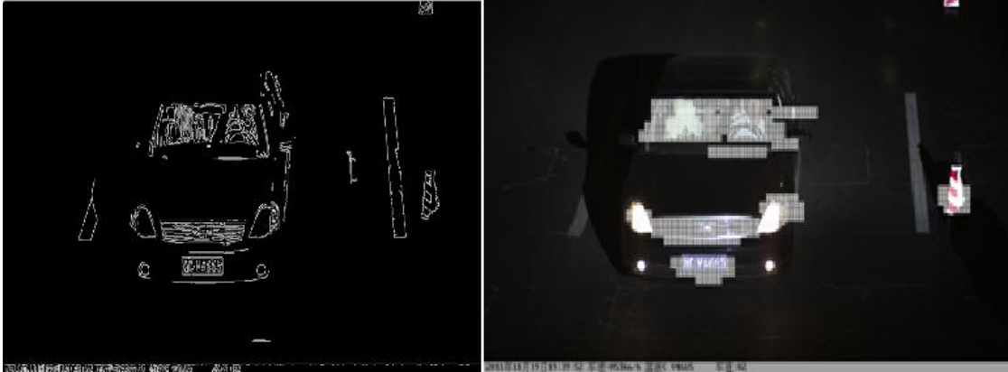
(Fig1. Edge image(left) and Scanned region(right))
