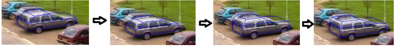
(Fig.15 Test on a SUV, Corresponding 3D model of(from left to right): First Generation, Second Generation, Generation 10, Converging Generation. The classification output type is SUV.)
