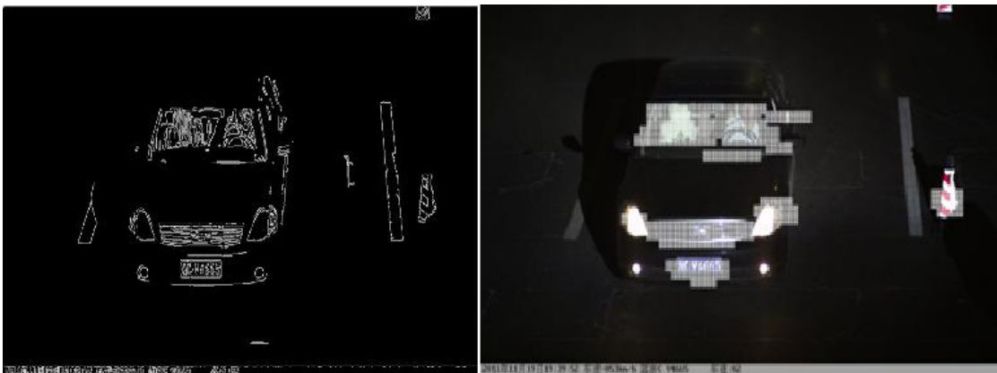
(Fig1. Edge image(left) and Scanned region(right))
